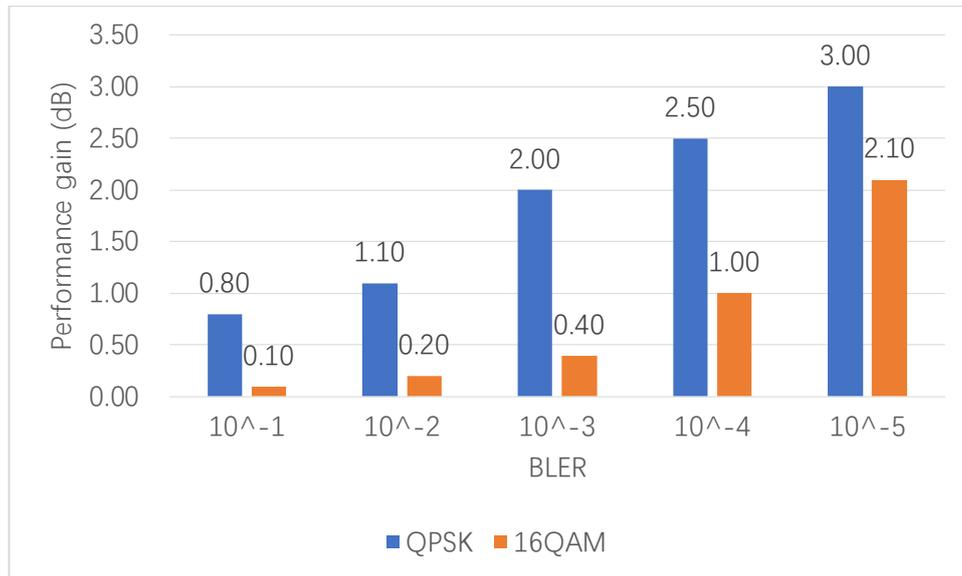
Figure 4-5 Performance Gains of Discrete Scheduling of Sub-carriers in Comparison with Continuous Scheduling of Sub-carriers
