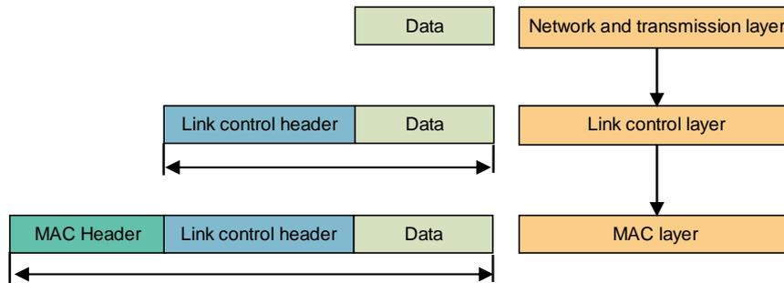
Figure 2-3 Data Encapsulation Process of the SLB System
