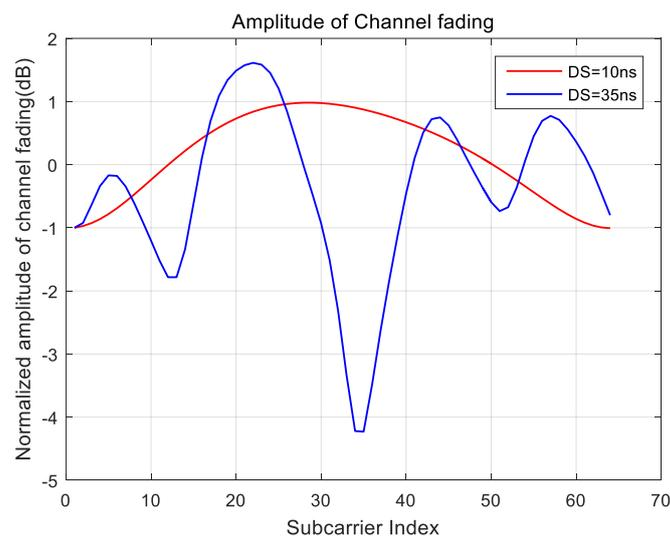
Figure 4-4 Fading Characteristics of Frequency Domain of In-vehicle Channels
