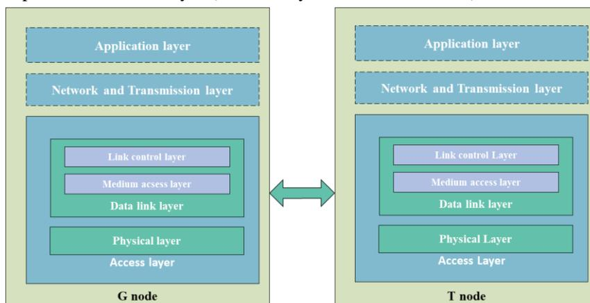
Figure 2-2 Architecture of Protocol Stacks of SparkLink System
