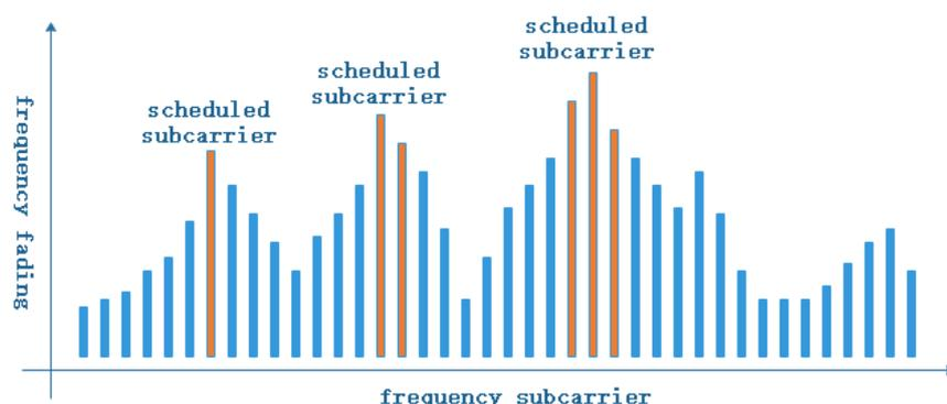
Figure 3-3 Schematic Diagram of Principles for Decentralized Scheduling
