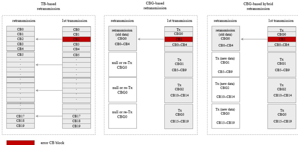
Figure 3-6 Schematic Diagram of HARQ Scheme
