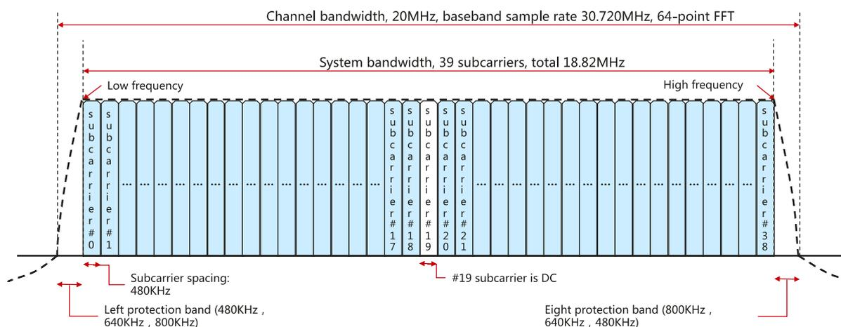
Figure 2-5 Division of Sub-carriers of SparkLink System (20MHz Channel)
