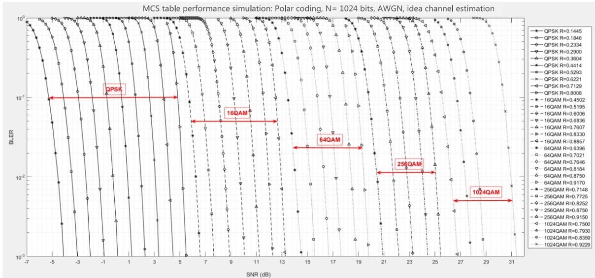
Figure 4-2 MCS Performance of Data Transmission with Large Packet/High Traffic (under AWGN Channel, Ideal Channel Estimation, N=1024-bit MCS0~31)
