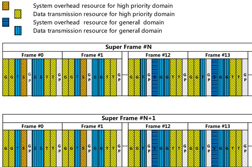
Figure 3-8 Schematic Diagram of Multi-domain Resource Coordination
