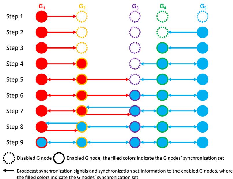
Figure 3-7 Schematic Diagram of Multi-node Synchronization in Time and Frequency Carriers
