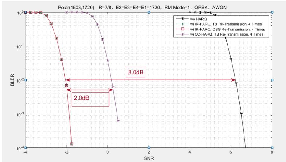
Figure 4-3 Comparison of Performance between CC/IR Retransmissions
