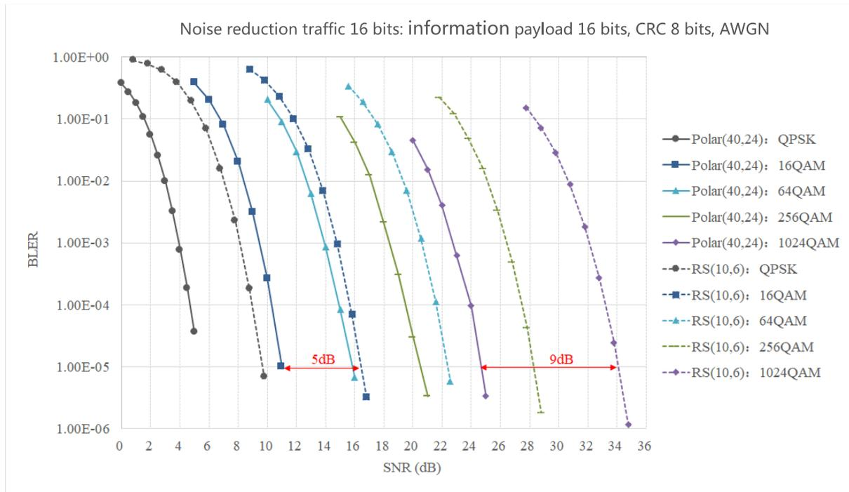
Figure 4-1 Comparison of Performance between Polar Code and RS Code under AWGN Channel (Number of Information Bits is 16-bit)
