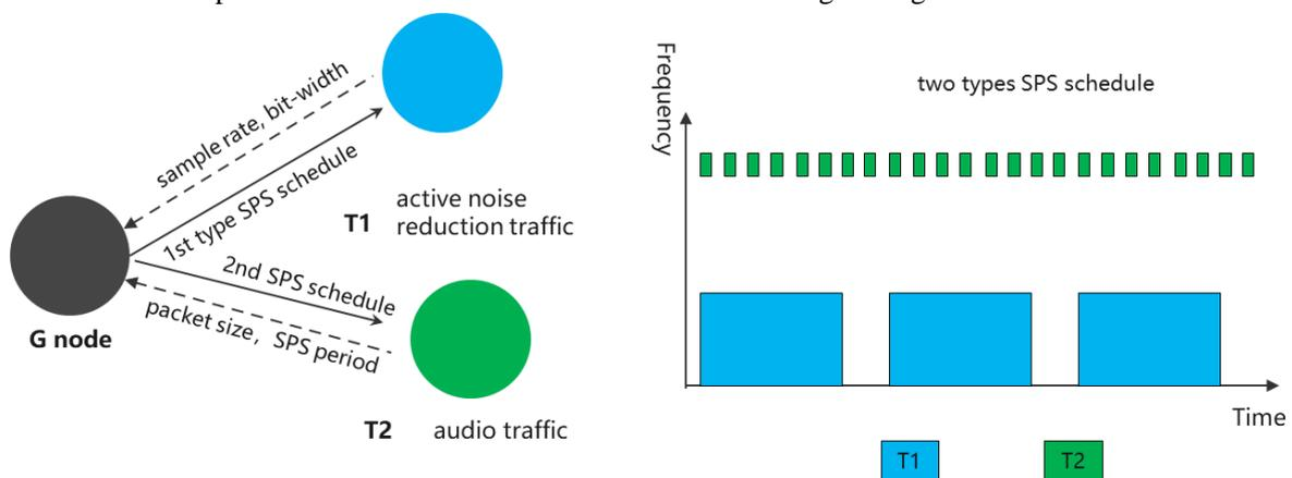
Figure 3-2 Fine Granularity Scheduling and Traffic Intelligent Scheduling of SLB System
