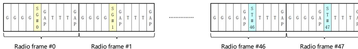
Figure 2-6 Superframe Structure of SparkLink System
